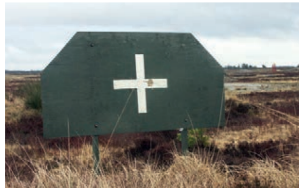
Stationary Armour Target (SAT) Capable of 136 kg (300 lbs) lift. Corresponds to target size 5 x 2.5 m in winds up to 15 m/s (35 mph).
