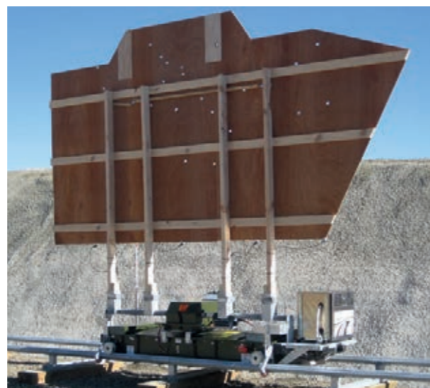
Moving Armour Target (MAT) Capable of 136 kg (300 lbs) lift. Corresponds to target size 5 x 2.5 m in winds up to 15 m/s (35 mph).
