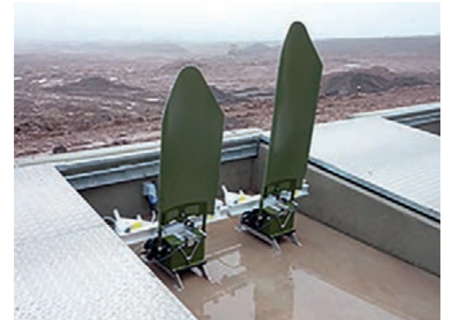
LOMAH 700 For stationary and moving infantry targets. Detection area 4 x 3 m (width x height).
