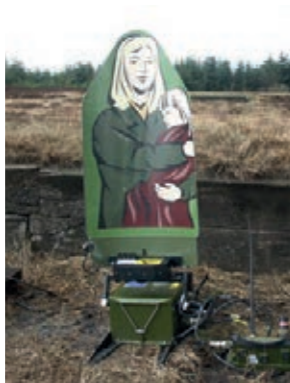
Swivel Target – Reaction shooting and friend vs enemy discrimination. Swivel includes the multi-target holder capability.
