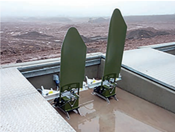
LOMAH 700 For stationary and moving infantry targets. Detection area 4 x 3 m (width x height).
