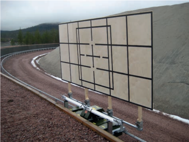
LOMAH 3000 For stationary and moving armour targets. Detection area 12 x 5 m (width x height).
