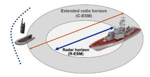
It provides wideband detection, classification, direction finding, geo-location, and monitoring of radio signals and other emitters of electromagnetic waves. Identification and tracking of emitters are supported as well as the integration to on-board systems like combat management systems.
