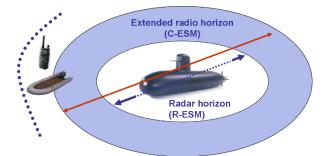
Together with other sensors the C-ESM & COMINT system provides longer emitter detection, interception and tracking range and therefore provides an earlier indication of activities and emerging events.
