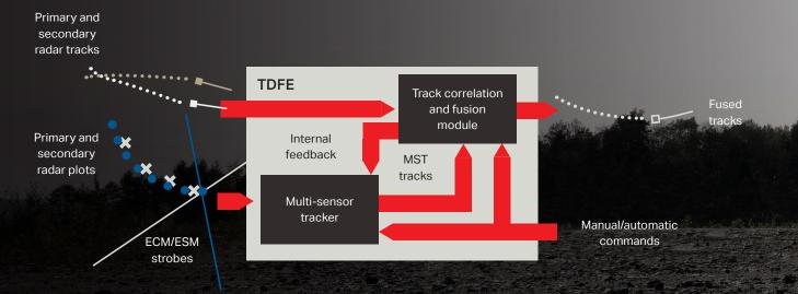
The TDFE is the result of more than 35 years' development of trackers and correlators. The system and its components are operational in several countries worldwide, with require-ments ranging from 1 sensor and 100 tracks to more than 100 sensors and 10,000 tracks. In fact, the upper number is unlimited.
