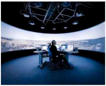
Saab's Remote Tower system uses a number of video, audio and other sensors to provide a continual, comprehensive view from the air traffic control tower. The data from cameras and other sensors is fed to a flight control centre, where air traffic controllers have complete control of all sensors and all lighting at the airport, along with integrated flight data, electronic flight strips and other air traffic control tools.
