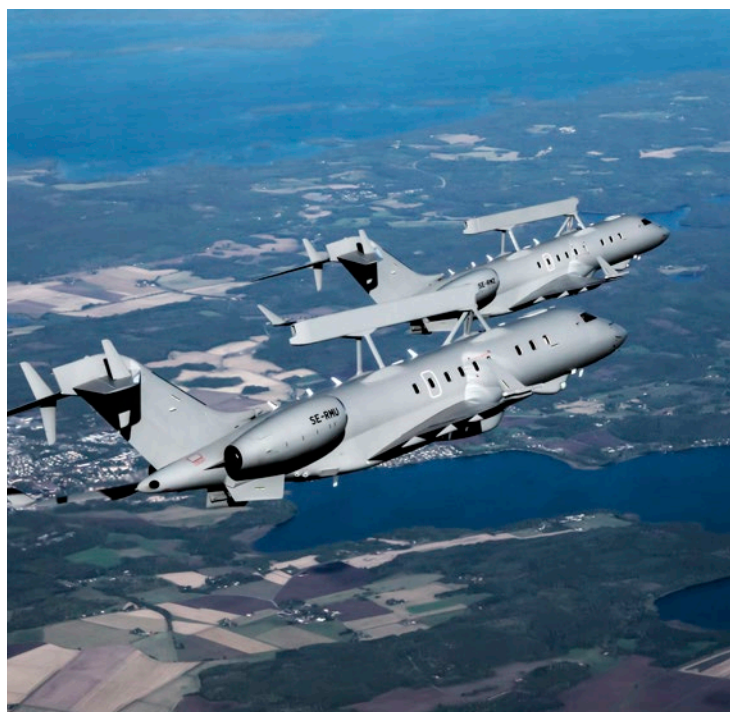
GlobalEye has a mix of modern active and passive sensors, providing long-range detection of objects in the air, at sea and over land.
