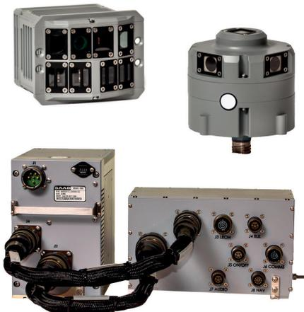
Naval Laser Warning System (NLWS) is capable of detecting and analyzing lasers in Blue Water and Littoral combat environments. This system provides vitally important situational awareness to the command team about the presence of laser emissions.
