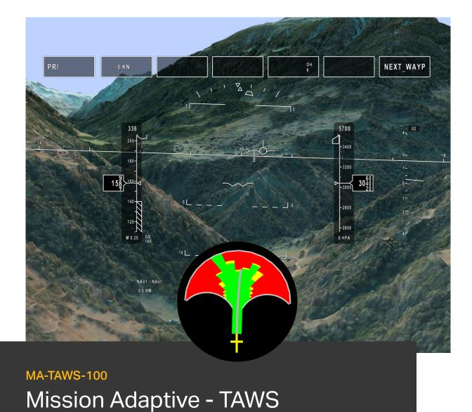
MA-TAWS-100 is one of Saab's next generation products providing airborne platforms with a performance based Terrain Awareness and Warning System (TAWS). MA-TAWS is designed to provide nuisance free Controlled Flight Into Terrain (CFIT) protection for missions in challenging terrain when mission requirements call for low-level altitude flights.
