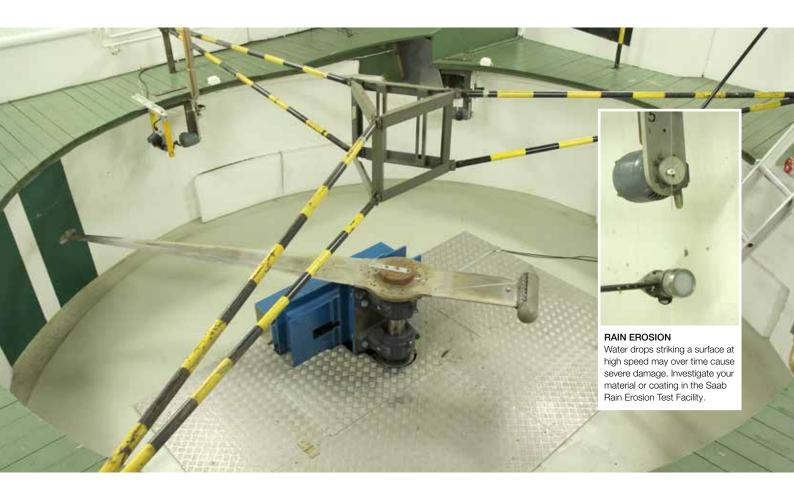
When water drops strike your product at high speed, materials or coatings you expected to be tough and enduring may over time get erosion damage. Cracks in coatings will increase the risk of such erosion.
