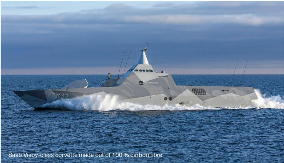
Saab Visby-class corvette made out of 100 % carbon fibre
