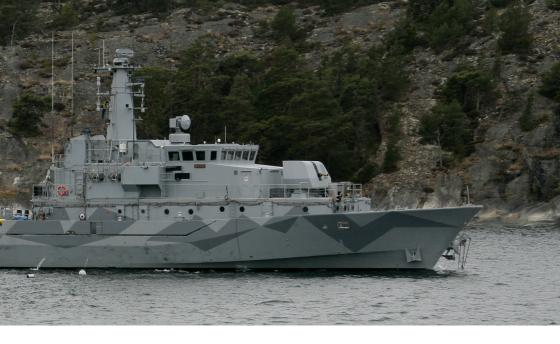
The main enhancements on MCMV 52 Koster-class include extending the Length Overall (LOA) by 5 m to 52.5 m. This creates more space for crew and systems, and improves sea-keeping and ensures a growth margin for the future. MCMV 52 Koster-class will keep the basic hull lines from the proven MCMV 47 Koster-class.
