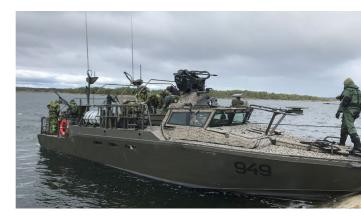
like Saab Trackfire, whilst a versatile and tough interior, combined with a strong bow ramp, ensure swift deployment onto unprepared beaches.
