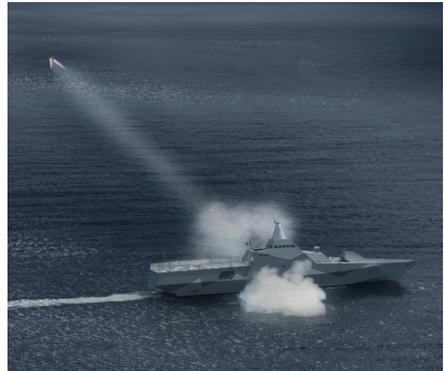
Visby-class corvette's all-composite carbon-fibre hull and superstructure is not only lighter than steel, but also comparable for fire resistance and ballistic properties, and superior to steel for vulnerability to blast and underwater explosions. In terms of life cycle costs, the carbon-fibre composite is entirely superior to steel and aluminium for fatigue. And the superior corrosion resistance reduces the platform lifecycle costs even further.
