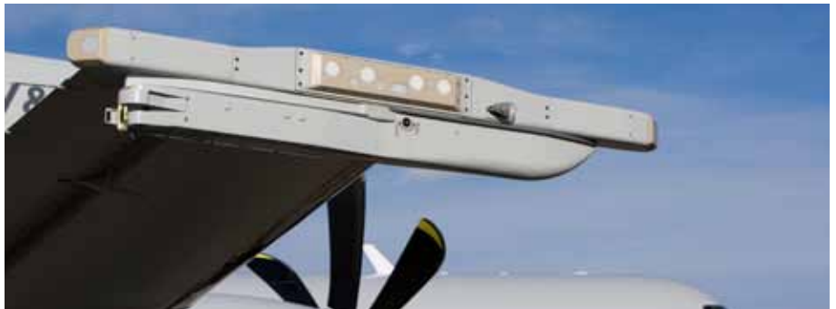
Radar Warning Sensors and Interferometer Antenna Array with BOL dispenser mounted below
