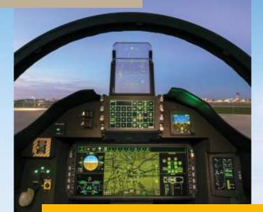
Digital Glass Cockpit Reconfigurable Large Area Display Open Architecture
